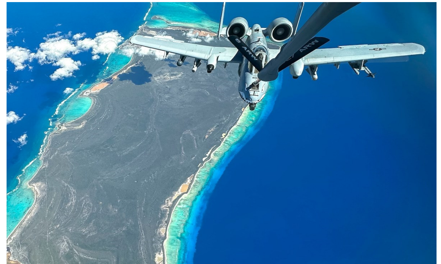
An A-10C Thunderbolt II aircraft receives fuel from a KC-135 Stratotanker over the Atlantic Ocean, Feb. 28, 2023.
